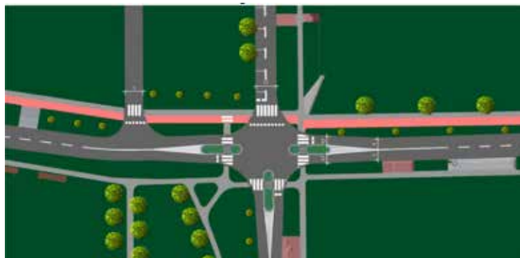
Figure 5. Reconstruction solution with pedestrian islands
